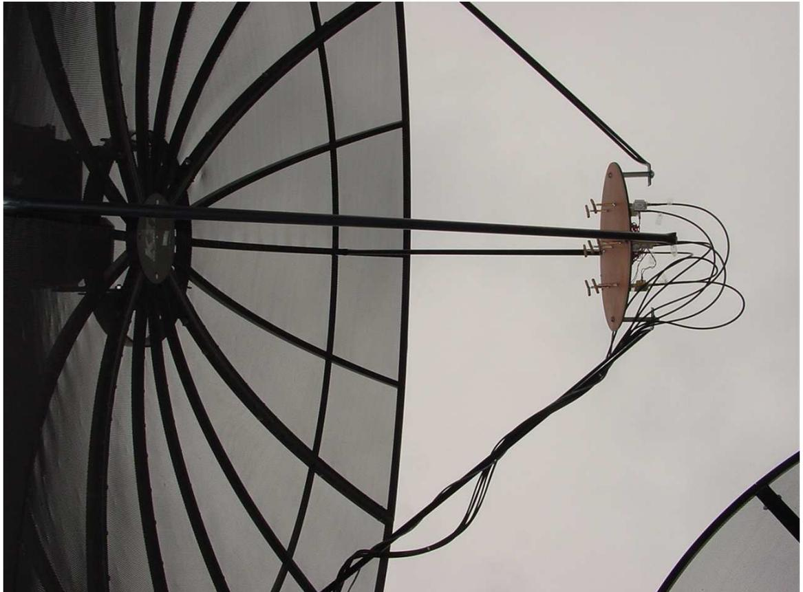
Figure 6.2: The array feed is mounted at the focal plane of a 3-meter reflector.
