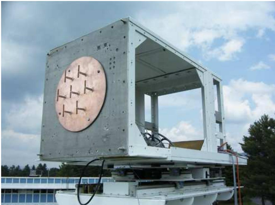
Figure 5.7: The seven-element array at the NRAO test range in Green Bank, WV. The incident electric field is co-polarized with the array elements and the rotation is along the H-plane.
