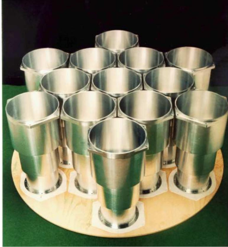
Figure 2.5: Picture of the Parkes 13-element waveguide array feed [30].
