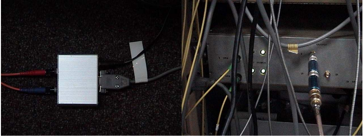
Figure 4.11: Left: RS-232 to optical fiber modem. Right: RF coax to optical modem. Input/Output 1 carries the signal from the 3.6 meter antenna.
