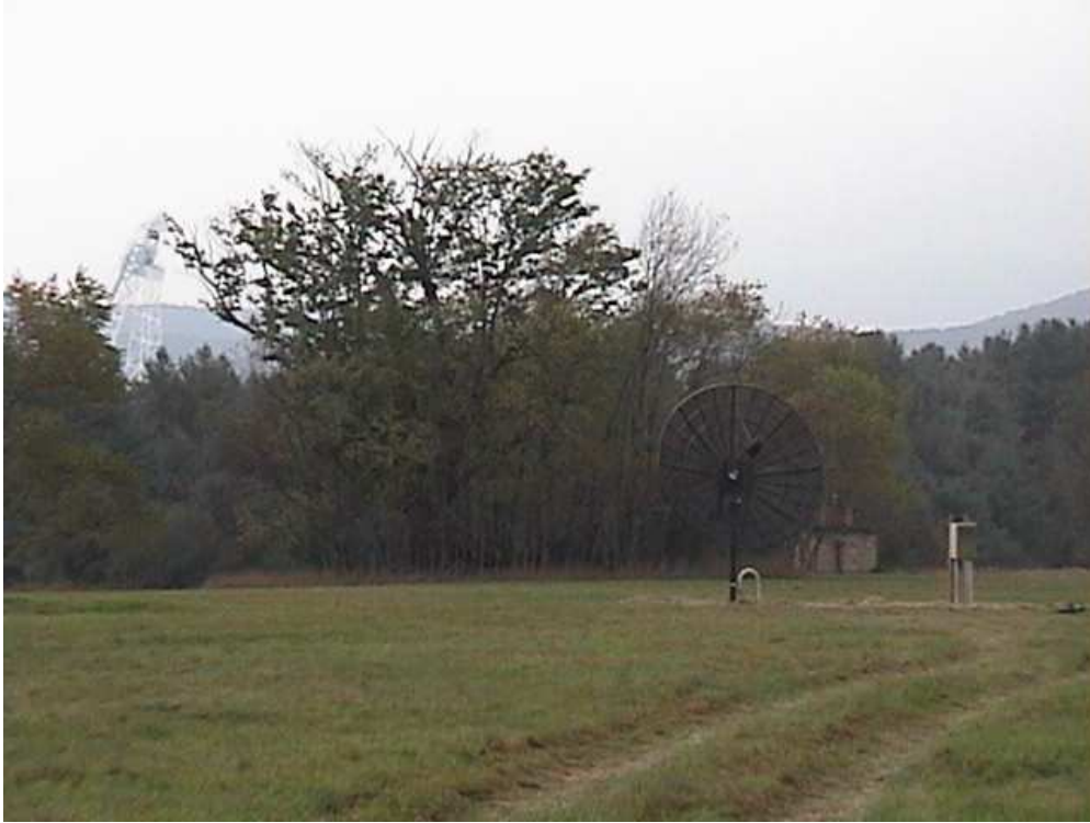
Figure 4.10: 3.6 meter reference antenna used for GBT interference cancellation tests. The weatherproof box to the right of the antenna houses the antenna control hardware and power supplies. Notice the GBT feed peeking over the trees.
