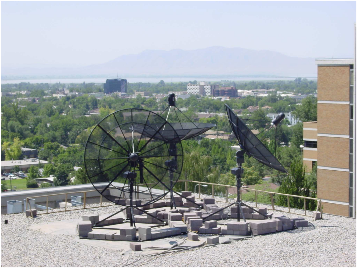
Figure 4.6: The BYU VSA in test configuration. The left antenna is pointed at a dipole antenna mounted on a tower. The signal transmitted by the dipole is either an FM sweep interfering signal or a “fake” astronomical source. The right antenna is tracking either a hydrogen source or a GLONASS satellite.
