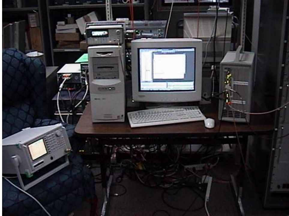
Figure 4.19: The DSP computer setup at Green Bank, WV. The spectrum analyzer on the chair at the left gave real-time analysis of the quality of the GLONASS reference signal. When the power received began to drop, I was able to recalibrate the reference antenna in order to maintain a consistently strong reference signal for the interference cancellation experiments. A power divider at the input to the DSP (at the right) sent a copy of the 3.6 meter signal to the spectrum analyzer. The signal generator sitting on top of the PC chassis served as the external DSP sample clock.
